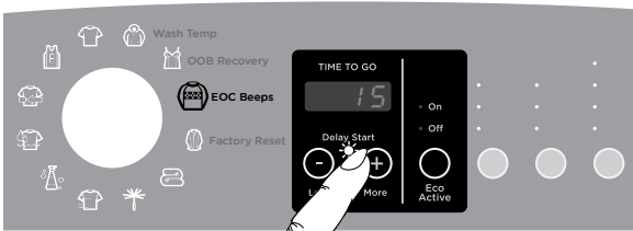
Modifying the number of beeps to signal the end of the cycle
